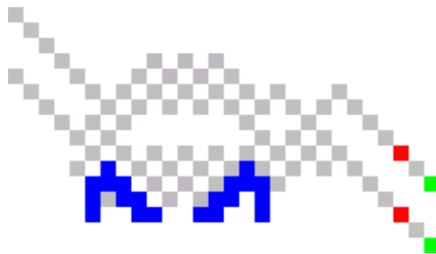
FIG. 12. A CAM8 implementation of an identity gate (composed of two switch gates back to back) and a crossover. The shaded squares are the wires, visualized every other time step. The signals have exited the circuit at the right.
